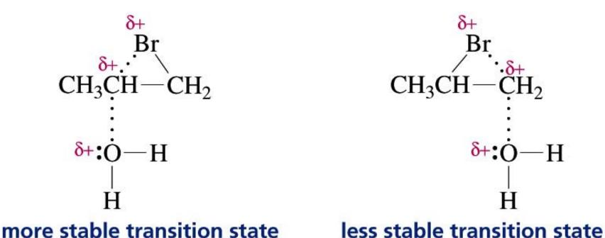
When water attacks the bromonium ion, it will attack the side that goes through the lower energy transition state.
